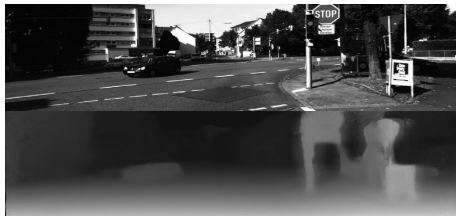
Fig. 1. Our depth prediction result on KITTI 2015. At top, single view input image. At bottom, our result of depth map prediction.
