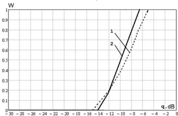
Fig. 8. Dependences of W(q) for "formant-like" noise (1 – received by results of tests (experiment with coherent texts); 2 – by an improved method)
