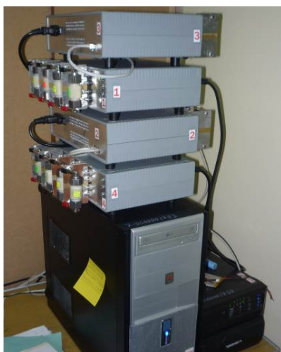
Fig. 3. Cell cycling system with four-cell modules.
